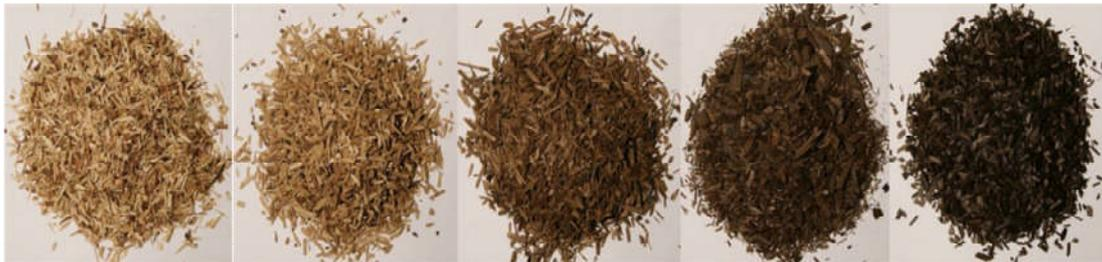
Figure 1 The change in colour of the biomass, from untreated (or raw) to biomass torrefied at increasingly higher temperatures and or residence times.
